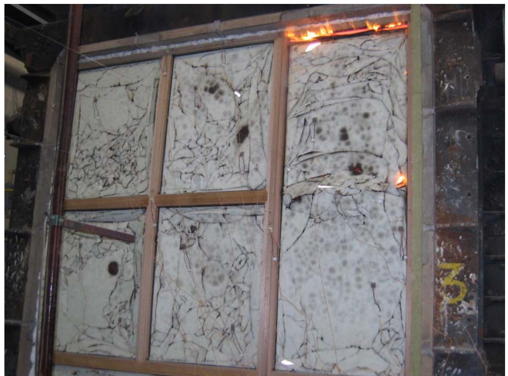
Showing the sustained flaming integrity failure of the specimen after 62 minutes of testing
