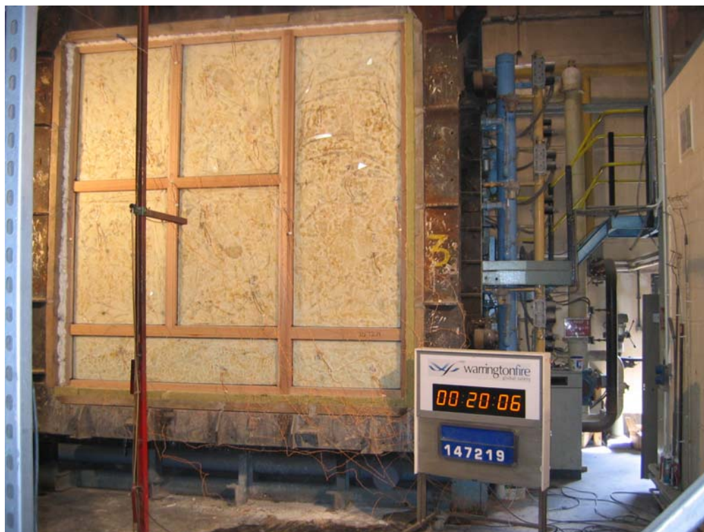
The unexposed face of the test construction during the test
