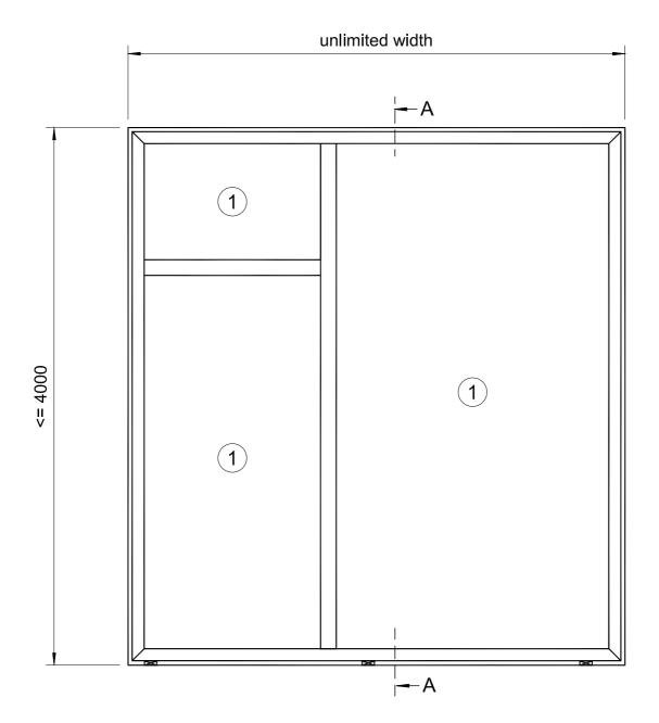
1 SGG CONTRAFLAM LITE 30 >= 13 mm, and SGG CONTRAFLAM LITE 30 IGU >= 23 mm, with the maximum dimension 1500 x 3000 mm
